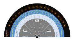
As shown in the figure, for a static goniometer tilt, the beam tilt can be incremented by a defined tilt step size and during the exposure time of the camera the beam tilt can sweep up a certain range. This ensures to completely scan the Fourier space.
